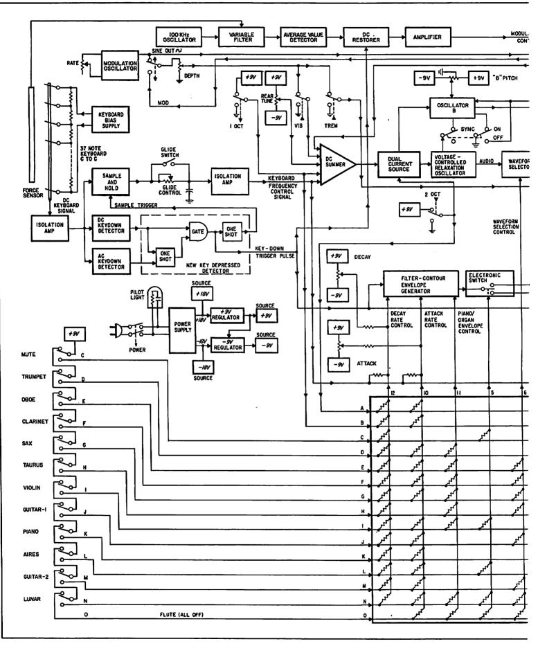
FIGURE 10-2 MINITMOOG BLOCK DIAGRAM
