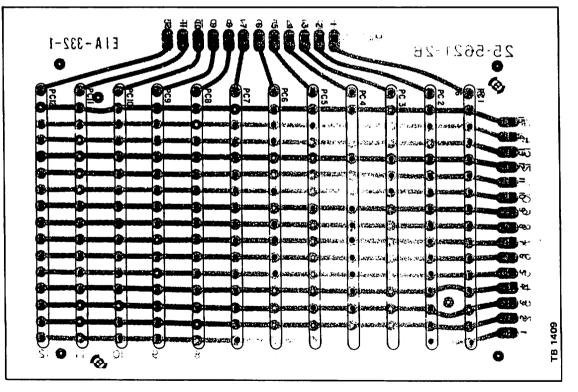
RESISTOR MATRIX PRINTED CIRCUIT BOARD ASSEMBLY
