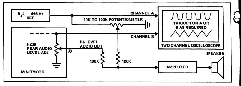
FIGURE 4-2 TWO CHANNEL OSCILLOSCOPE TEST SETUP FOR TUNING
