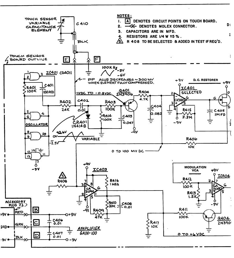
FIGURE 10-4 MINITMOOG TOUCH SENSOR BOARD ASSEMBY NO. 4 SCHEMATIC DIAGRAM
