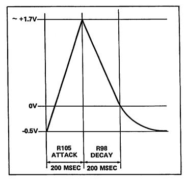
FIGURE 4-8 FILTER CONTOUR AT 020 SOURCE
