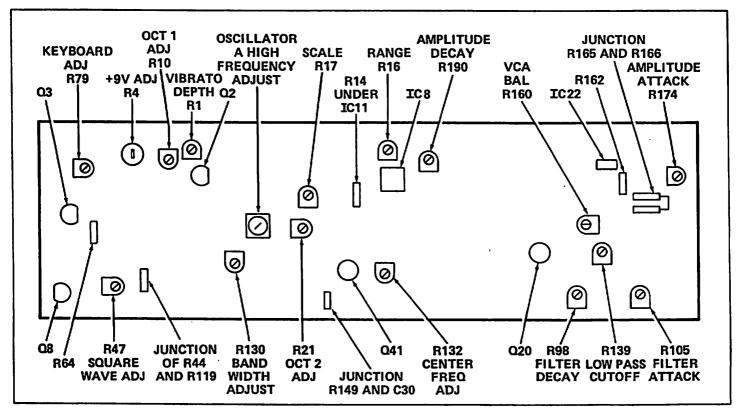
FIGURE 4-3 MAIN BOARD NO. 1 ADJUSTMENT CONTROLS AND OSCILLOSCOPE TEST POINT LOCATIONS
