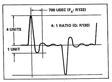
FIGURE 4-7 BAND PASS FILTER Q AND F<sub>C</sub> AT Q41 SOURCE
