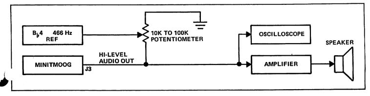
FIGURE 4-1 MINIMAL TEST SETUP FOR TUNING
