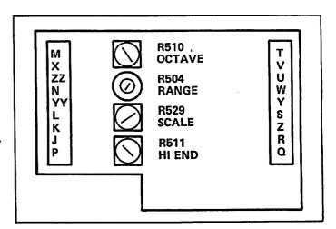
FIGURE 4-5 OSCILLATOR B TRIMPOT LOCATIONS (BOARD NO. 5)
