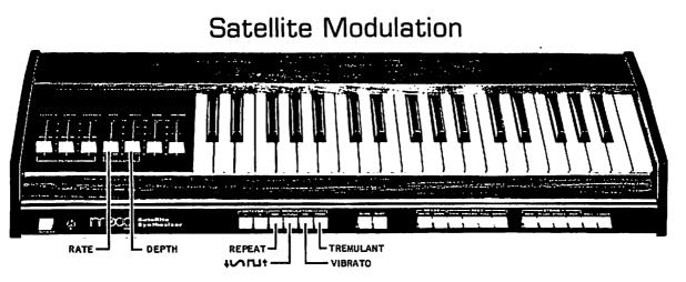
The four function tabs labeled MODULATION on the front of the unit provide a selection of modulation types. The two MODULATION slide controls on the slide control panel adjust the RATE and DEPTH of modulation.
