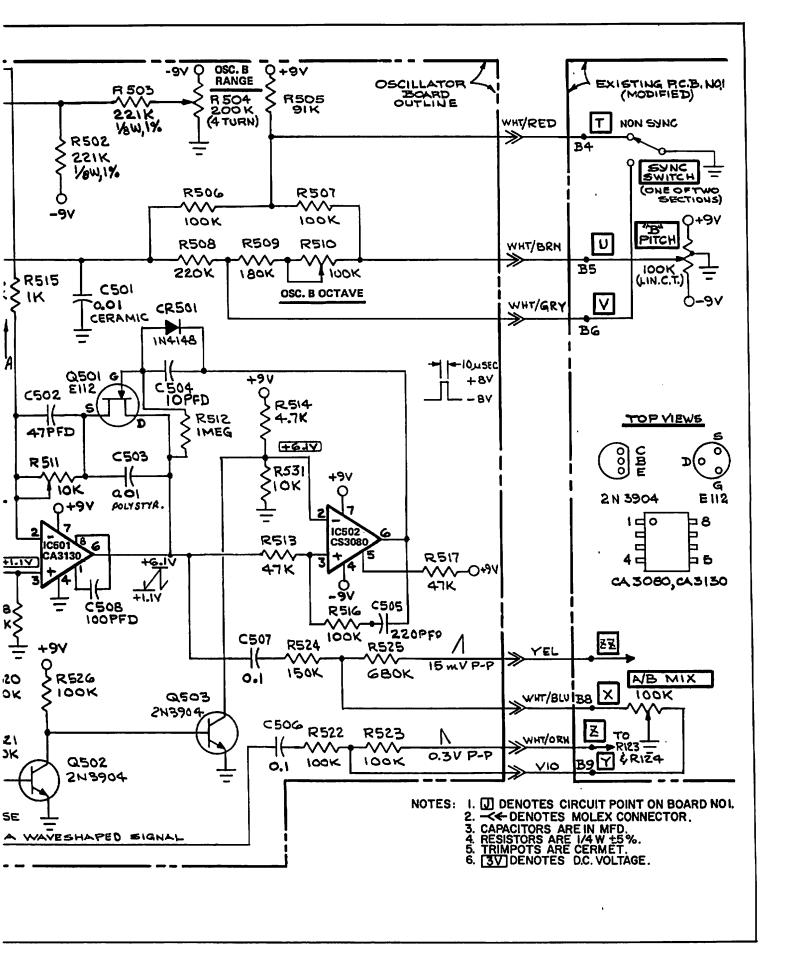
FIGURE 10-5 MINITMOOG OSCILLATOR BOARD ASSEMBLY NO. 5 SCHEMATIC DIAGRAM
