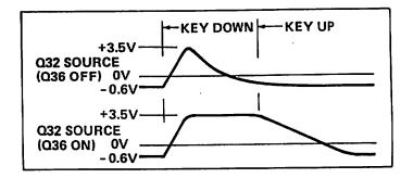
FIGURE 2-5 SOURCE VOLTAGE OF Q32
