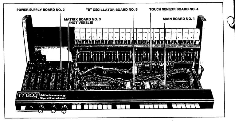
FIGURE 3-1 MINITMOOG PRINTED CIRCUIT BOARD LOCATIONS (INSIDE VIEW)
