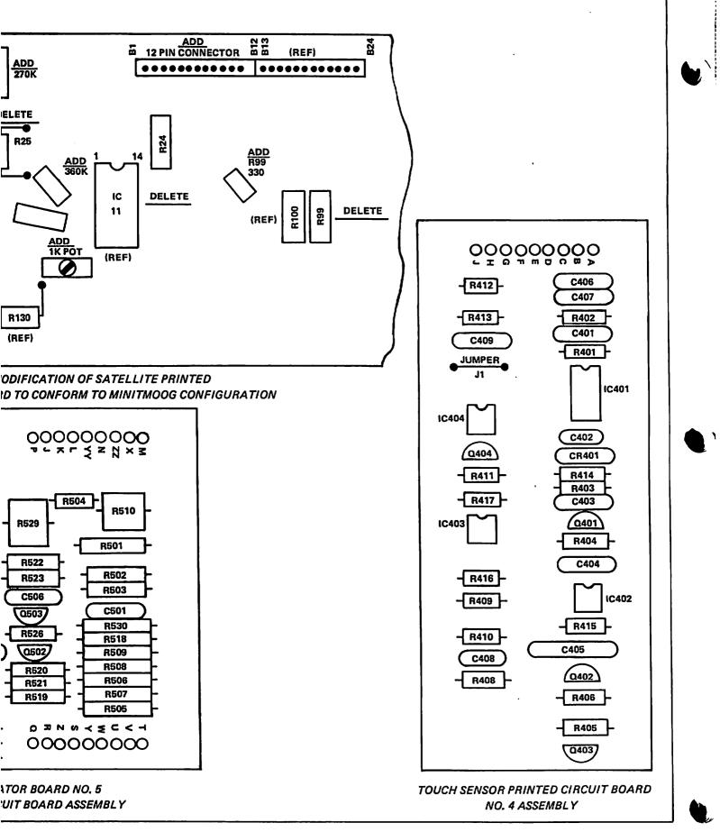
FIGURE 10-3 MINITMOOG PRINTED CIRCUIT BOARD ASSEMBLIES
